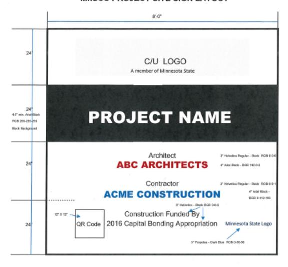
Site Sign shall be 8' x 8', 3/4" Exterior grade/MDO Plywood (4) - 2' Sections vertically:
